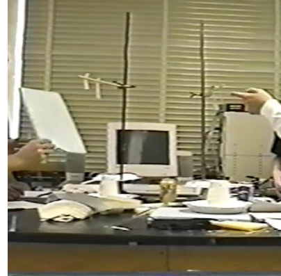
Fig. 1 Laboratory set-up showing ring stand and dowel rod with hanging strips of cellophane tape
